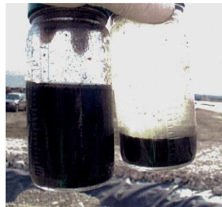
**Geotube® containers were periodically measured for fill height (left). *In situ* sediment sample (left) compared to chemical conditioned sediment.**
