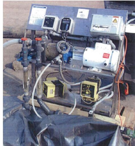
**Geotube® containers in operation and filtrate being sampled (left). The photo on the right shows the WaterSolve WSLP-2400 polymer make-down unit in operation.**
